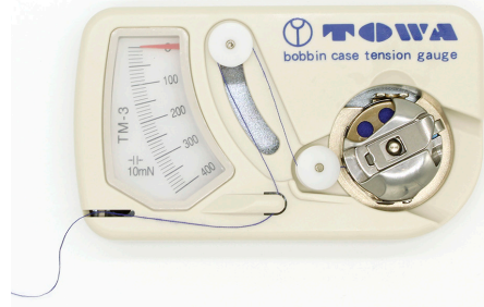
TOWA Gauge Use to check your bobbin tension
